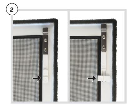
Turn the lower part of the plastic fitting 90° so that the fitting moves upwards and becomes resilient. The springy fittings should be upwards on the frame.
