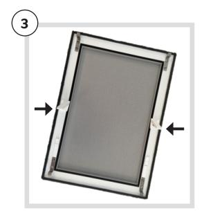
Grab the plastic handles in the center of the mosquito net frame, angle the frame and bring it out through the window frame. Then push the frame upwards against the aluminum edge of the window frame. Then put the frame in the correct position with the lower fittings around the aluminum edge.
